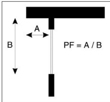
To take this exception, the projection factor for the shading device is calculated and this number is then matched with the corresponding multiplier. Refer to **SHGC Multiplier Table** below. This multiplier is then applied to the rated SHGC of the glazing component that is being installed with a
