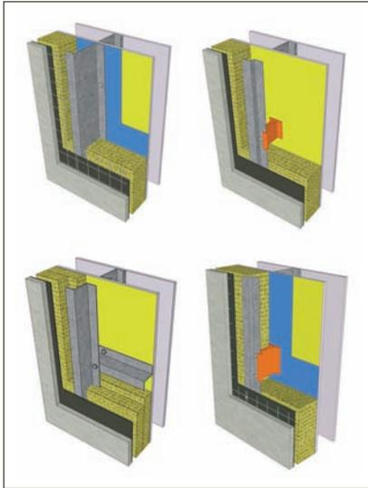
None of these wall assemblies can be considered to have a continuous insulation layer, and therefore, determination of the U-value requires looking up default values in WSEC Chapter 10 tables (if possible) or using the Zone Method of calculation.
